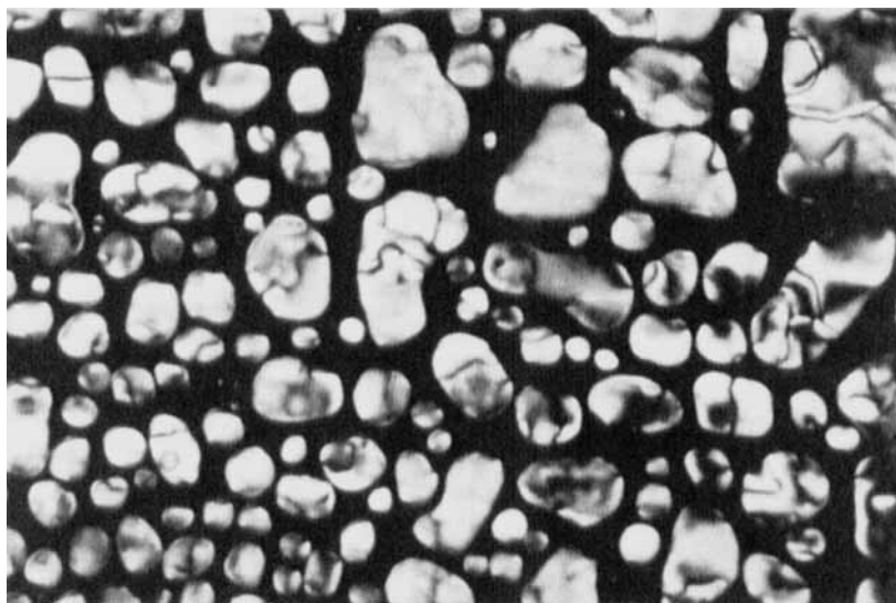
Fig.2 : Nematic droplets at the clearing point. Monomer where n = 6
